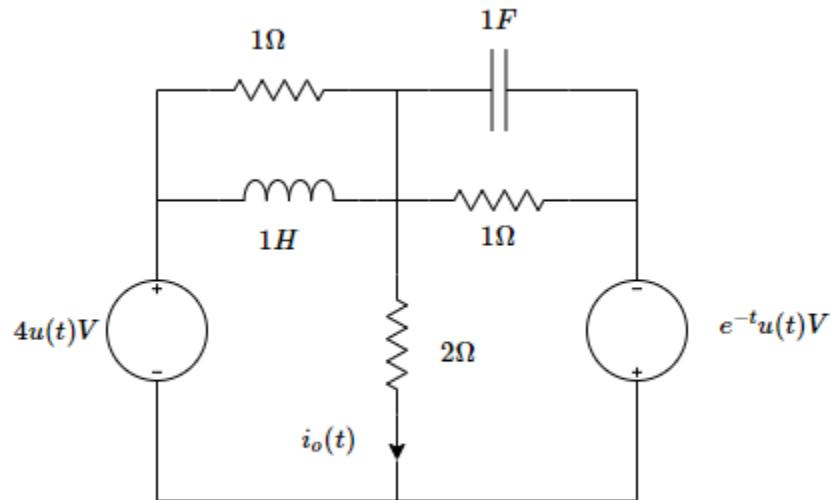
1. Determine the  $s$ -domain representation of this circuit and re-draw the circuit (3pts)
