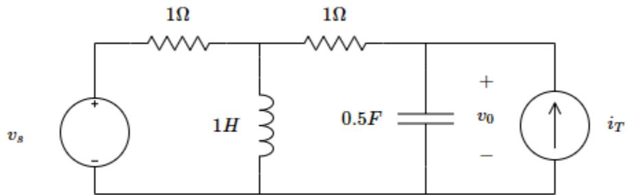
It is required to find  $v_0(t)$  when the voltage and current source are respectively given by:  $v_s(t) = K_1 u(t)$  and  $i_T(t) = K_2 \delta(t)$ . Assume no initial conditions on the capacitor and inductor
