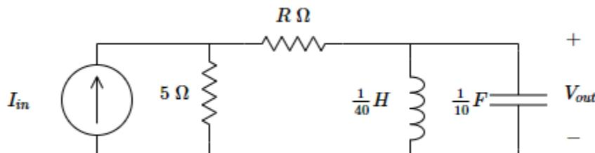
(Hint: Convert the current source to a voltage source and back to a current source)
